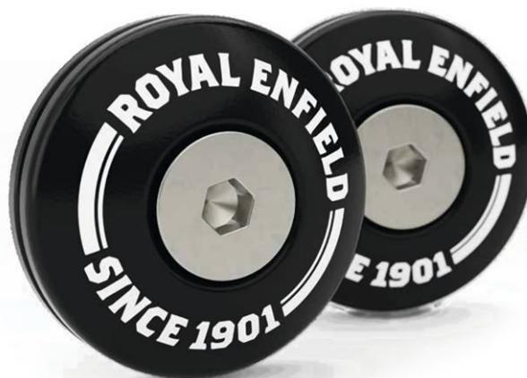
Subtly style your motorcycle with these handlebar finishers. They are machined from billet aluminium and anodized for a long life.
