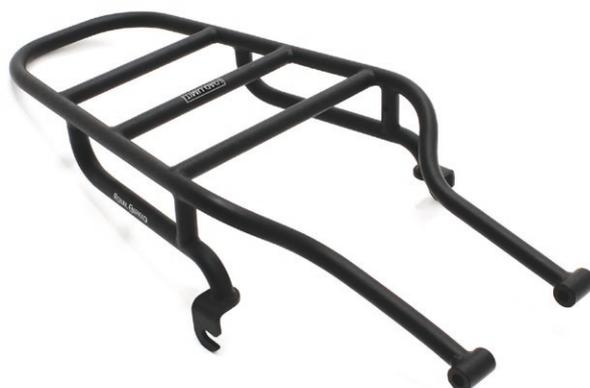
Manufactured from 16mm diameter mild steel tubing. Black powder coated to give a durable, corrosion resistant finish. Royal Enfield branded.
